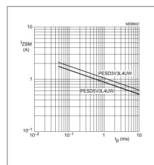
Fig.2 Non-repetitive peak reverse current as a function of pulse time (square pulse).
